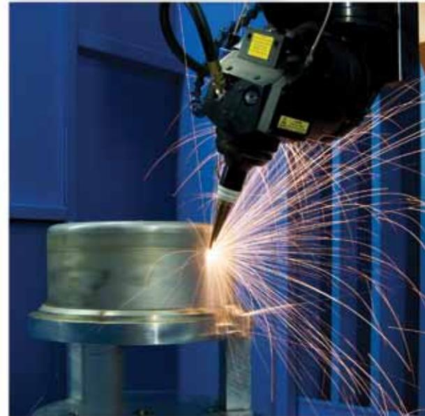
*High speed drilling on the fly with a CL50k Nd:YAG laser using LASERDYNE exclusive OFC (Optical Focus Control), BTB (BreakThrough Detection), and CylPerf programming at normal, minor, shallow, and compound angles.*
