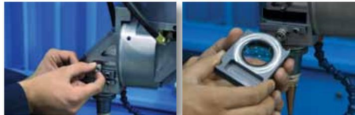
*Quick change lens and cover slide drawers allow an operator to make foolproof changes in seconds.*
